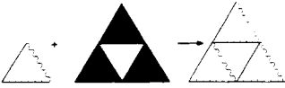
Figure 2. To construct our fractal lattices, copies of the initiator ‘atom’ are connected according to the generating tie scheme to yield the second-order lattice.
